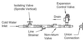
Note: a combined isolating valve/non-return valve/line strainer may be used.
